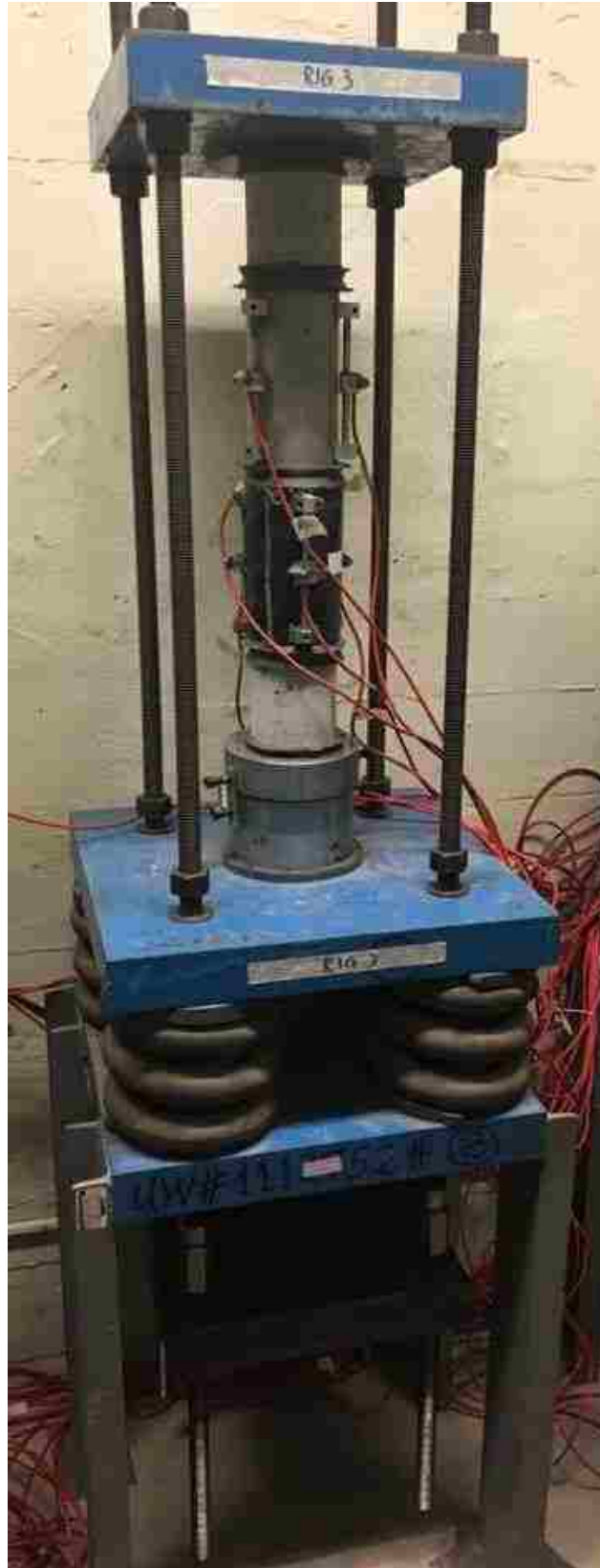
Figure 3.5 A Loaded Creep Rig in the Lab
